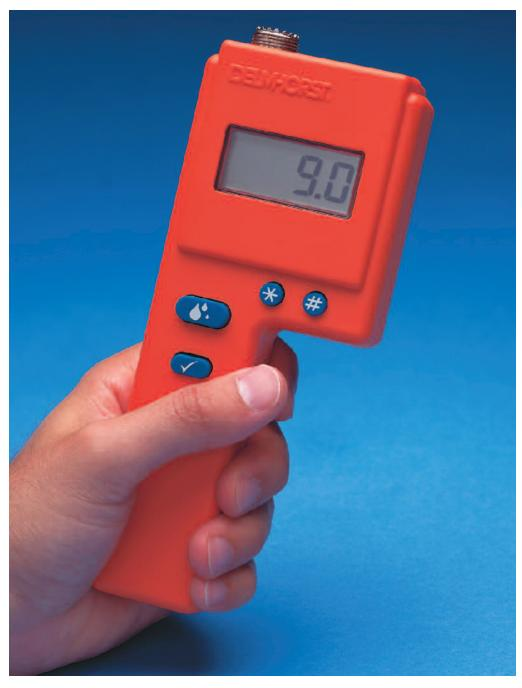
A moisture tester is a valuable tool during the ginning process and when buying or selling cotton. Cotton ginned at the appropriate level of moisture produces the longest and strongest fibers.
