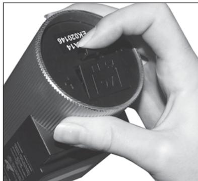
The battery box is located on the bottom of the tester. Open the box by pushing the locking lever over the battery symbol as shown in the picture (see image) and replace the battery.
